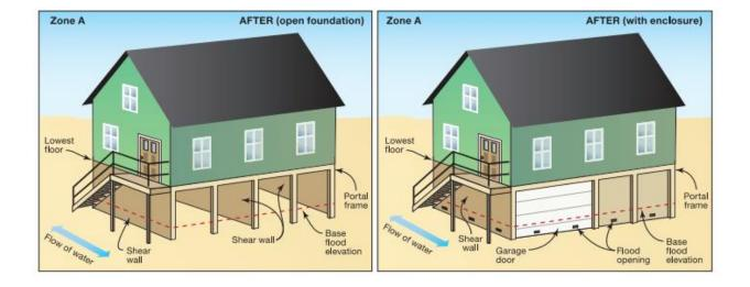
Figure 1. Before (2.5-story house at-grade) and after (1.5-story house with NFIP-compliant open foundation or compliant enclosure below the BFE) of a house in Zone A with the lower floor converted using a shear wall and portal frame foundation system. FEMA; Reducing Flood Risk and Flood Insurance Premiums for Existing Residential Buildings in Zone A.
